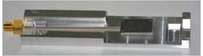
Fig. 6. Photograph of proof-of-concept version of integrated antenna.
