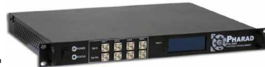
can switch any of four input optical signals carrying RF signals to any of four output ports, as required in a particular application. The Photonic Cross-Connect operates independently of the frequencies of the RF signals being transported over fiber. In addition to providing real-time creation and reconfiguration of the photonic signal paths, the Photonic Cross-Connect includes continuous optical power monitoring to ensure reliable operation of the entire system.
