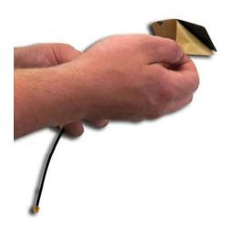
**Step 4:** Connect the antenna to the equipment via the RF connector.
