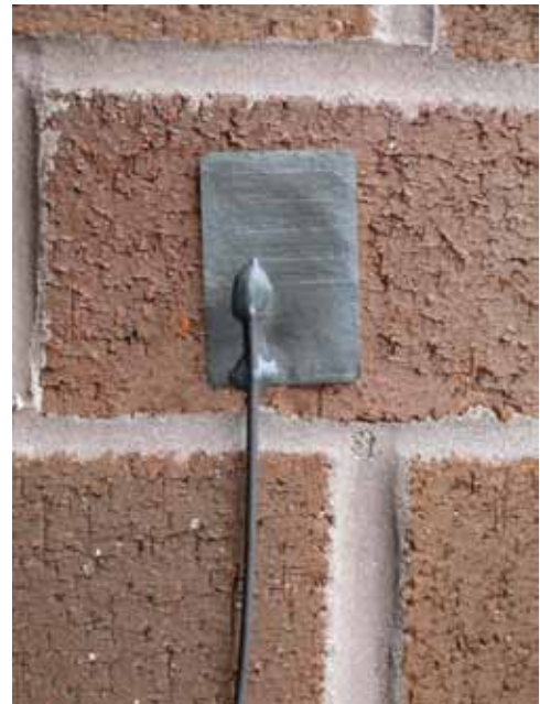
Pharad's peel & stick appliqué antennas can adhere to the outside of car windows, a building, and plastic enclosures
