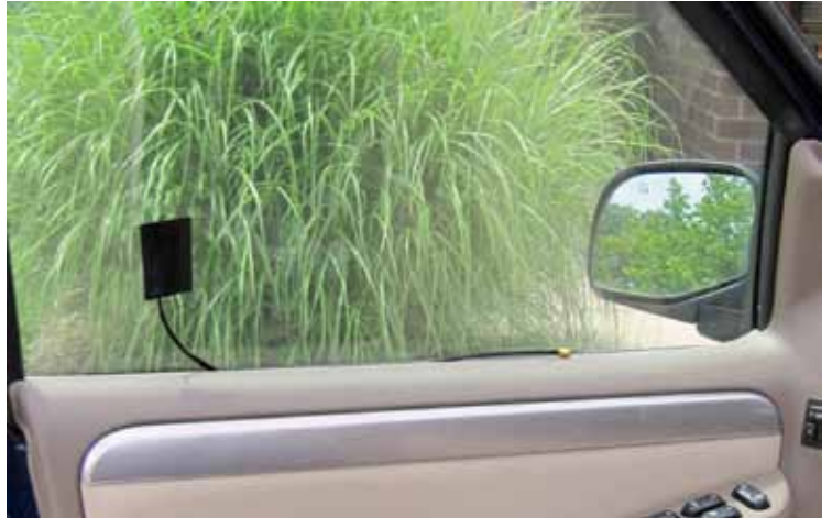
Pharad's peel & stick appliqué antennas can adhere to the outside of car windows, a building, and plastic enclosures
